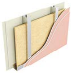
Option 2 2 x 12.5mm British Gypsum Fireline plasterboard each side, single 100mm stud, 1 x ISOVER 50mm APR 1200 quilt to cavity. O/A width 150mm.
