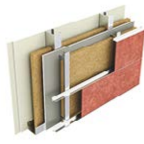
Option 3 Type EC1i: Two layers of minimum 12.5mm British Gypsum Fireline plasterboard, stud with ISOVER 50mm APR 1200 between, sheathing board, Rockwool Duo Slab Insulation, ventilated rainscreen.
