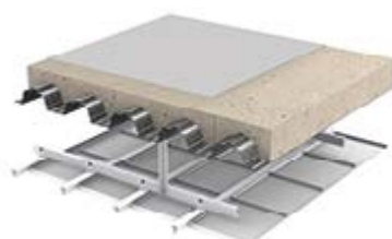
Option 6 Minimum 160mm deep concrete slab (80mm minimum), 5mm Collecta Rubberform, MF ceiling with 1 x 15mm British Gypsum Soundbloc.
