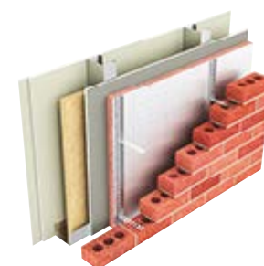
Option 2 Type EC1i: Two layers of minimum 12.5mm British Gypsum Fireline plasterboard, stud with ISOVER 50mm APR 1200 between, sheathing board, Kingspan K15 Insulation, 50mm cavity, brickwork.
