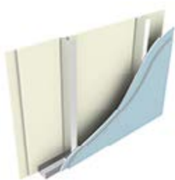
Option 1 2 x 15mm British Gypsum SoundBloc soundboard plasterboard each side, single 100mm stud. O/A width 160mm.
