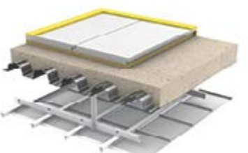
Option 7 (Scotland) Minimum 160mm deep concrete slab (80mm minimum), Collecta Screedboard 30, Metsec MF ceiling with 1 x 15mm British Gypsum Soundbloc.
