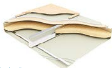
Option 3 Type F9: Three layers of 12.5mm British Gypsum Fireline plasterboard, resilient bars, joists with 1 x ISOVER 50mm APR 1200 quilt to cavity, 15mm plywood, 19mm British Gypsum Plank, 70mm Collecta Deckfon acoustic battens, 18mm V313 chipboard.
