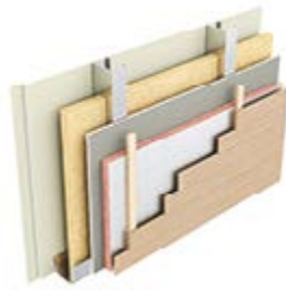
Option 4 Type EC1i: Two layers of minimum 12.5mm British Gypsum Fireline plasterboard, stud with ISOVER 50mm APR 1200 between, sheathing board, Kingspan K15 Insulation, battens, timber cladding.
