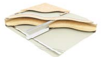
Option 5 Type F9: Three layers of 15mm British Gypsum Fireline plasterboard, Metsec RB565 resilient bars, joists with 1 x ISOVER 50mm APR 1200 quilt to cavity, 15mm plywood, 19mm British Gypsum Plank, 70mm Collecta Deckfon acoustic battens, 18mm V313 chipboard.
