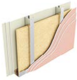
Option 4 3 x 15mm British Gypsum Fireline plasterboard each side, single 100mm stud, 1 x ISOVER 50mm APR 1200 quilt to cavity. O/A width 190mm.
